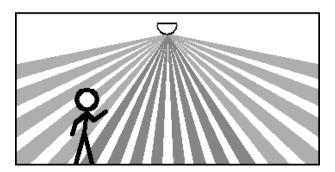
At a distance closer to the sensor, even slow movement can be detected. As the movement is away from the sensor, the space between the zones of sensitivity increases, and therefore the amount of motion required to trigger the device increases.
