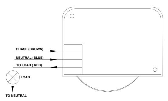
Note: Use 0.75 Sq.mm.flexible wires for connections (Phase, neutral & load)
